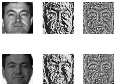
Figure 4.14: The effects of LBP preprocessing: first column - the original images under different illumination intensities; second column - the original LBP preprocessing; third column - the simplified LBP preprocessing. The face size is 64 by 64.
