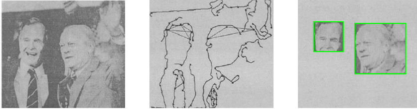
Figure 2.2: Example of edge-based face detection: original image, grouped edges, and detected faces [58].
