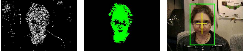
Figure 2.1: Per-pixel skin classification, blob growing, and detected face [118].
